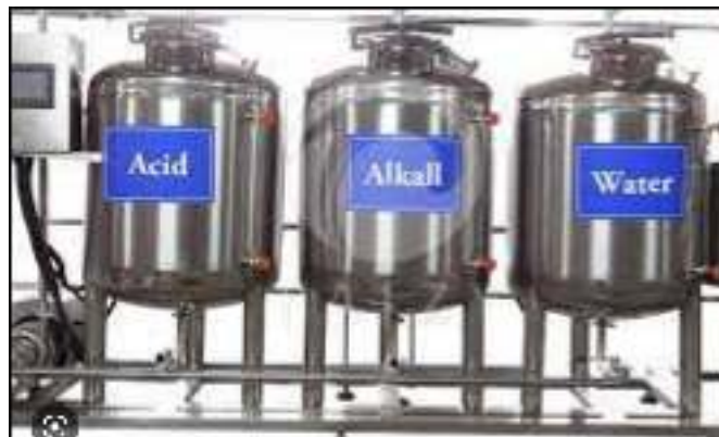
Figure 5.3: CIP with detergent
