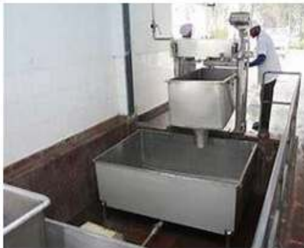
Figure 1 16: Milk Dump (Drop) Tank
