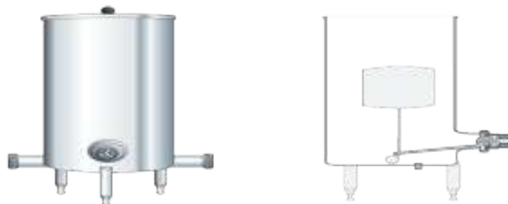
Figure 4.7 Balance tank for constant inlet pressure to the pump.
