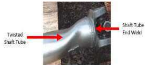
Figure 2-9 Inspection of Driveshaft Tube
