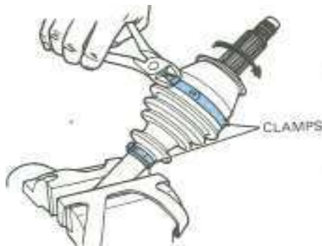
Figure 2-4 Cutting boot clamp
