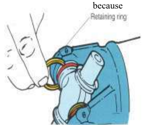
Figure 2-2 Sometimes snap rings go on the inside of the yoke.
