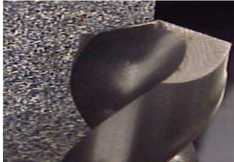
Figure:3.6 Line up the end of the web with the corner of the wheel.
