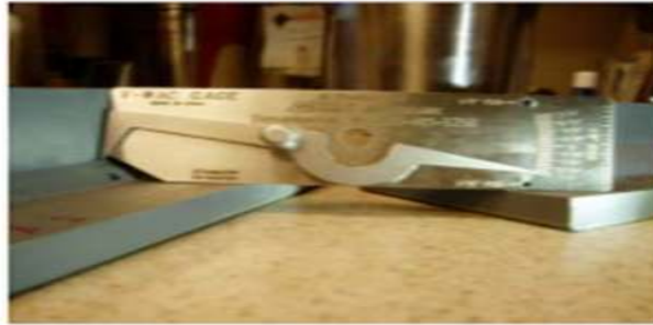
Figure 3.12. Bridge cam gauge
