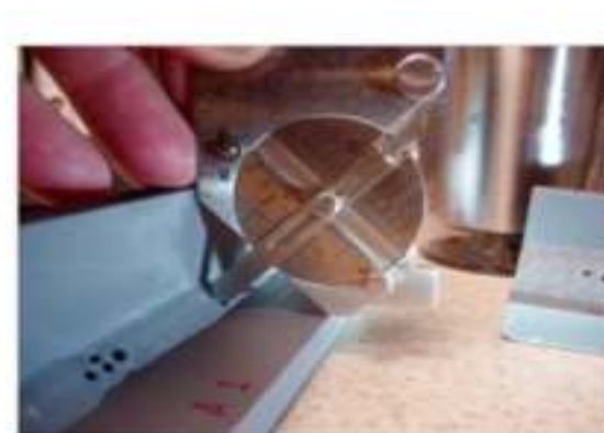
Figure 3.11. Throat measurement with cam gauge
