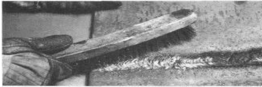
Fig.5.1 After chipping, brush the weld with a wire brush
