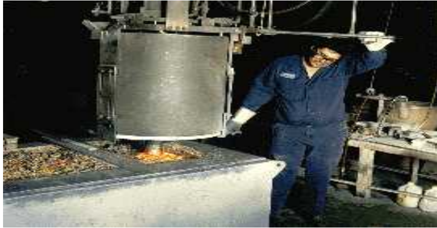
Fig.3.9. Phenol formaldehyde binders are employed for thick sections of CI, steel castings
