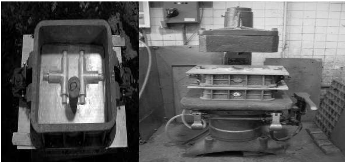
Fig. 3.10 Left; semi-automatic Machine, Right; core pattern p
