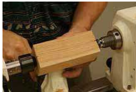
Fig. 2.56 Exercise blank mounted on lathe
