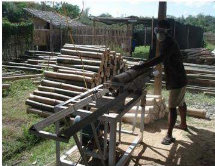
Figure 2:- Producing slats with the use of a twin-blade saw.
