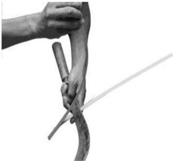
Step 7: Bend the bamboo a little as shown in the image to control the split
