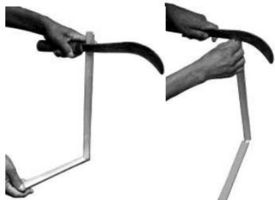
Step 4: Split this further to smaller width as required
