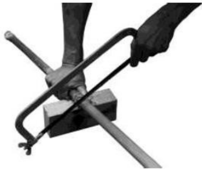
Step 1: Cut the bamboo to the required size with the help of a hacksaw/handsaw
