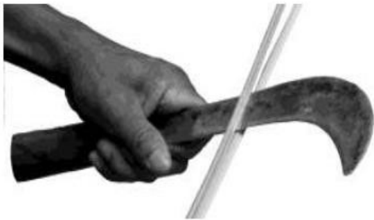
Step 5: Split bamboo further for uniform width
