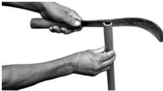
Step 3: Split the bamboo into two halves
