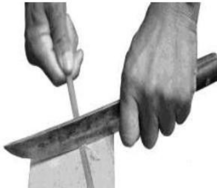
Step 8: Keep the thin sliver between the knife and a wooden plank as shown and pull the sliver to clean it further
