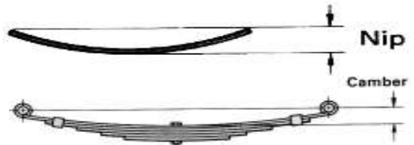
Figure 1-7 Parts of leaf spring
