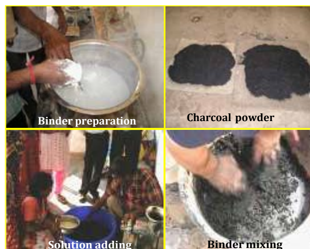
Figure 11. Preparing and mixing binder with charcoal powder
