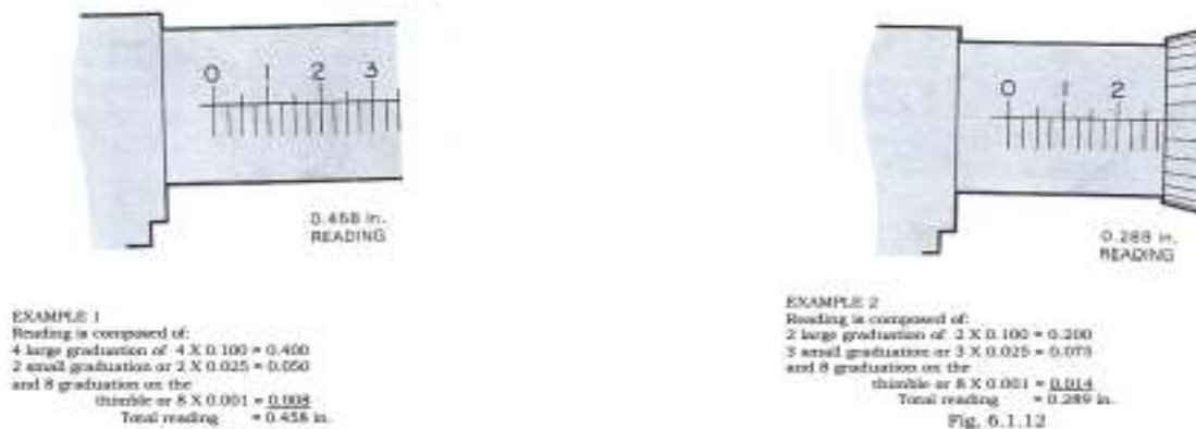
Figure 2.6 Reading micrometer
