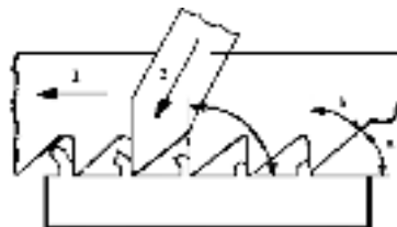
Figure 3.13 Hacksaw tooth setting
