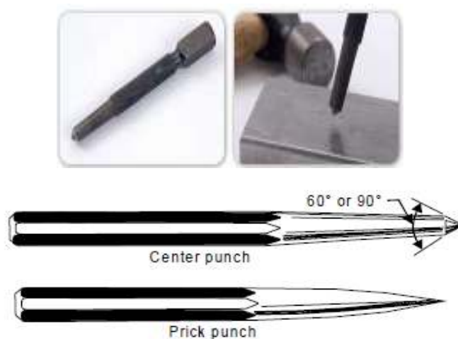
Figure 2.19. Center punch, and the punch in use.
