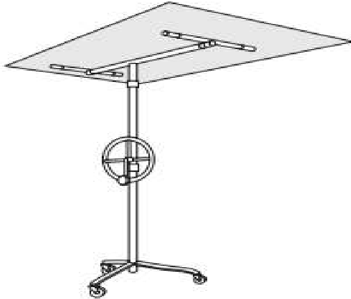
FIG:1.32. Panel Lift
