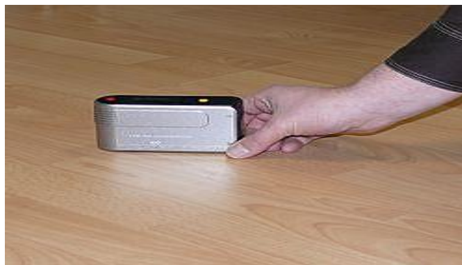
Fig 4.3 Gloss is typically measured with a gloss meter.
